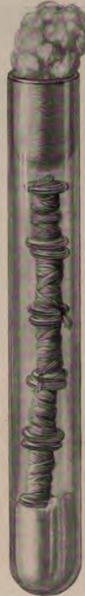
FIG. 8.—ROLLS OF STERILIZED SILK THREADS ON GLASS BOBBINS PRESERVED IN STOUT GLASS IGNITION TUBES. \frac{3}{4} ORDINARY SIZE.
